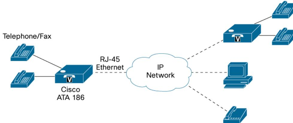
The Cisco ATA 186 allows you to connect analog telephones and faxes to an IP telephony network.
